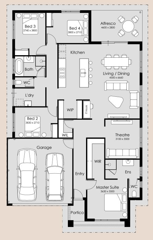
Overall Width – 12.19m Overall Length – 19.39m Min Block Width – 15m Min Block Length – 25m Total Area – 214.78m<sup>2</sup>
