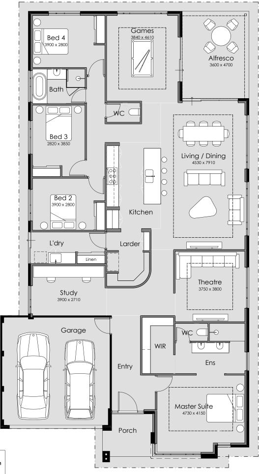
OVERALL WIDTH- 13.39m OVERALL LENGTH- 24.29m MIN BLOCK WIDTH- 15m MIN BLOCK LENGTH- 30m TOTAL AREA- 287.57m<sup>2</sup>
