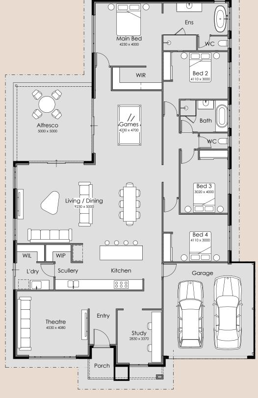
Overall Width – 15.39m Overall Length – 24.29m Min Block Width – 17m Min Block Length – 35m Total Area – 305.40m<sup>2</sup>
