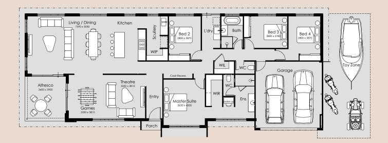
Overall Width – 26.09m Overall Length – 10.79m Min Block Width – 28.59m Total Area – 253.66m<sup>2</sup>
