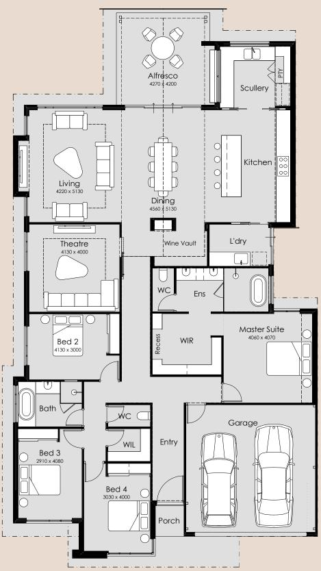
Overall Width – 13.89m Overall Length – 24.75m Min Block Width – 15m Min Block Length – 30m Total Area – 289.23m<sup>2</sup>
