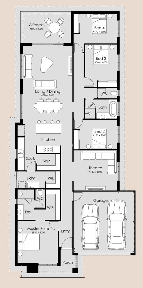
Overall Width - 11.39m Overall Length – 24.69m Min Block Width - 12.50m Min Block Length - 30m Total Area - 240.57m<sup>2</sup>
