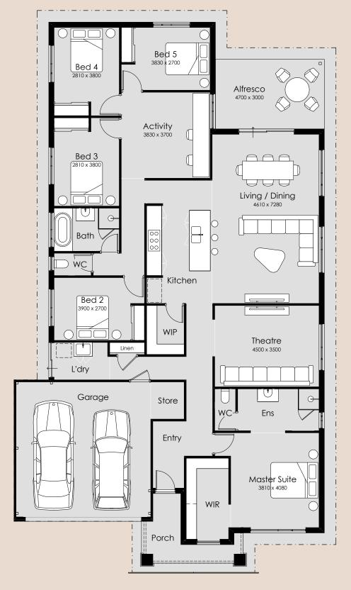
Overall Width – 13.39m Overall Length – 23.39m Min Block Width – 15m Min Block Length – 25m Total Area – 266.78m<sup>2</sup>
