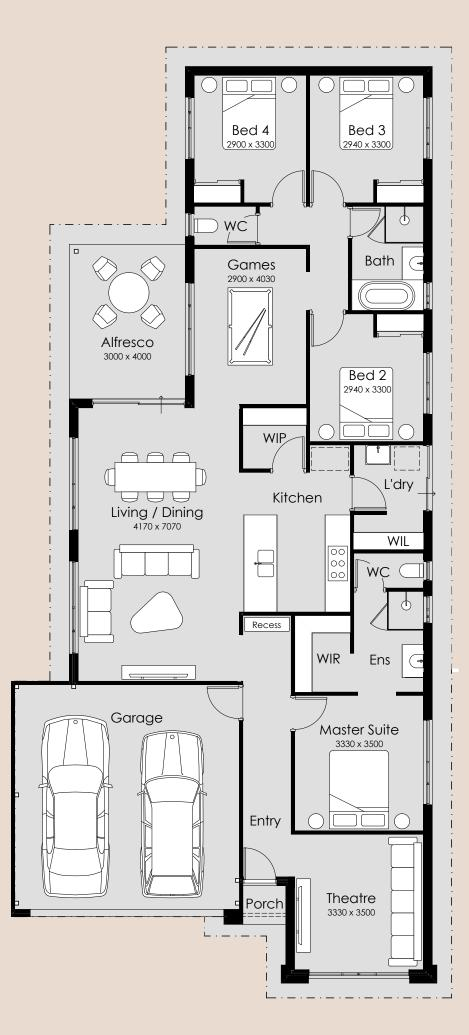
Overall Width – 11.01m Overall Length – 23.71m Min Block Width – 12.5m Min Block Length – 25m Total Area – 208.21m<sup>2</sup>
