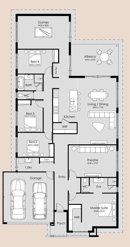
Overall Width – 13.89m Overall Length – 25.89m Min Block Width – 15m Min Block Length – 30m Total Area – 286.98m<sup>2</sup>
