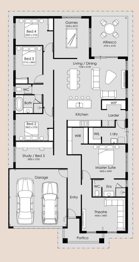
Overall Width - 12.09m Overall Length - 22.99m Min Block Width - 15m Min Block Length - 25m Total Area - 259.60m<sup>2</sup>
