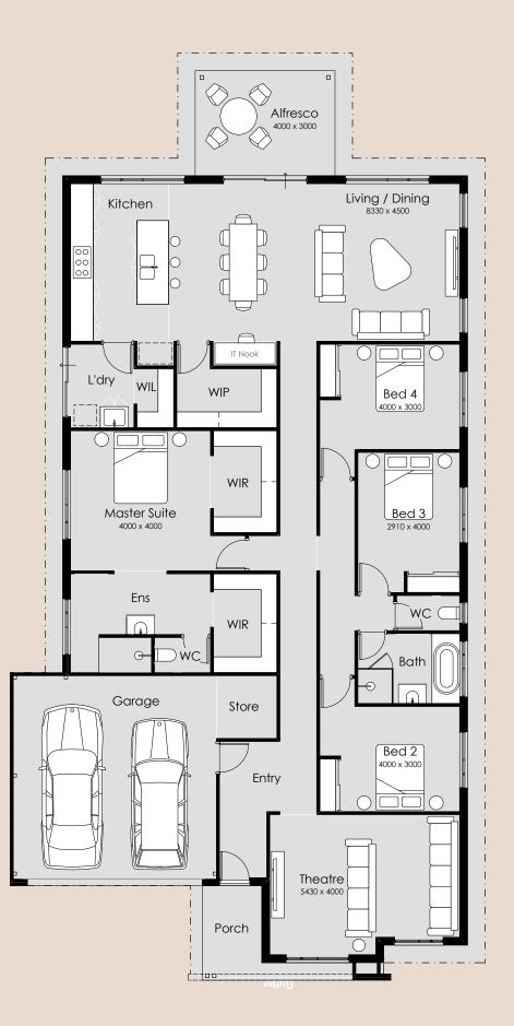
Overall Width – 13.09m Overall Length – 25.85m Min Block Width – 15m Min Block Length – 30m Total Area – 274.34m<sup>2</sup>
