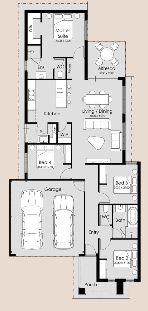
Overall Width – 10.39m Overall Length – 22.49m Min Block Width – 10.50m Min Block Length – 25m Total Area – 177.54m<sup>2</sup>
