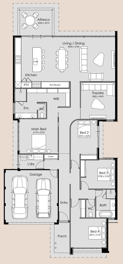
Overall Width – 12.39m Overall Length – 26.66m Min Block Width – 12.5m Min Block Length – 30m Total Area – 256.40m<sup>2</sup>
