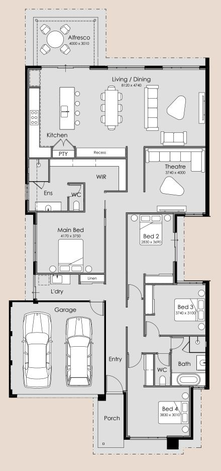
Overall Width - 12.39m Overall Length – 26.70m Min Block Width - 12.5m Min Block Length - 30m Total Area - 256.35m<sup>2</sup>
