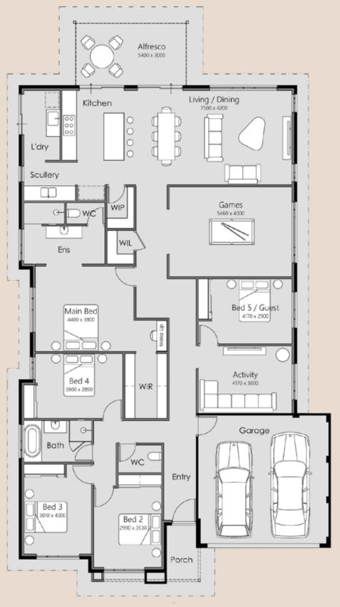
Overall Width – 13.89m Overall Length – 25.05m Min Block Width – 15m Min Block Length – 30m Total Area – 285.46m<sup>2</sup>
