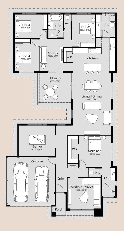
Overall Width – 13.39m Overall Length – 24.59m Min Block Width – 15m Min Block Length – 30m Total Area – 268.34m<sup>2</sup>
