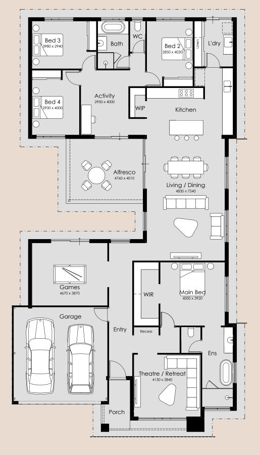
Overall Width - 13.89m Overall Length - 25.59m Min Block Width - 15m Min Block Length - 30m Total Area - 294.38m<sup>2</sup>
