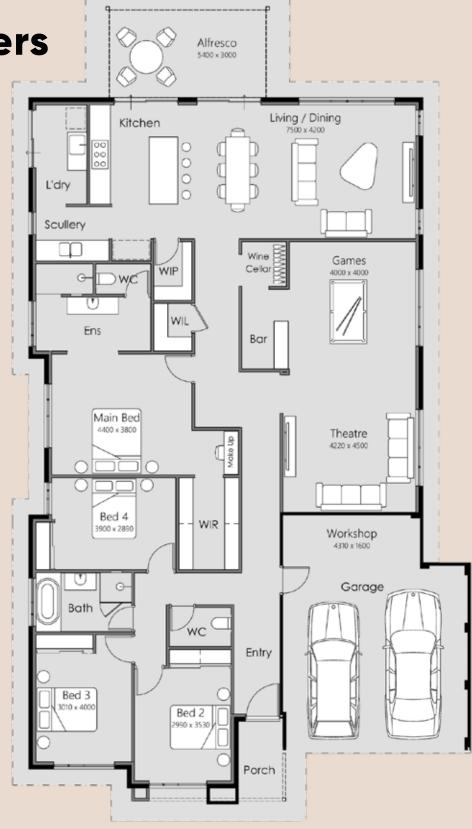
Overall Width - 13.89m Overall Length - 25.05m Min Block Width - 15m Min Block Length - 30m Total Area - 285.46m<sup>2</sup>
