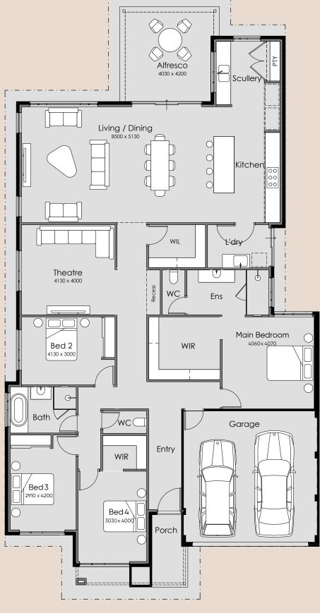
Overall Width - 13.89m Overall Length - 24.75m Min Block Width - 15m Min Block Length - 30m Total Area - 282.95m<sup>2</sup>
