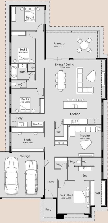
Overall Width – 13.89m Overall Length – 26.99m Min Block Width – 15.00m Min Block Length – 30.00m Total Area – 293.87m<sup>2</sup>
