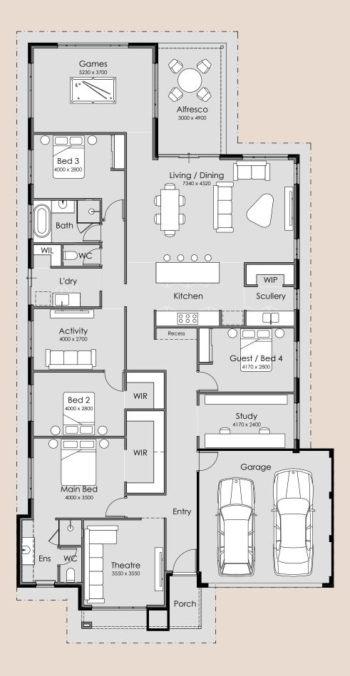
Overall Width – 13.89m Overall Length – 25.79m Min Block Width – 15m Min Block Length – 30m Total Area – 288.77m<sup>2</sup>
