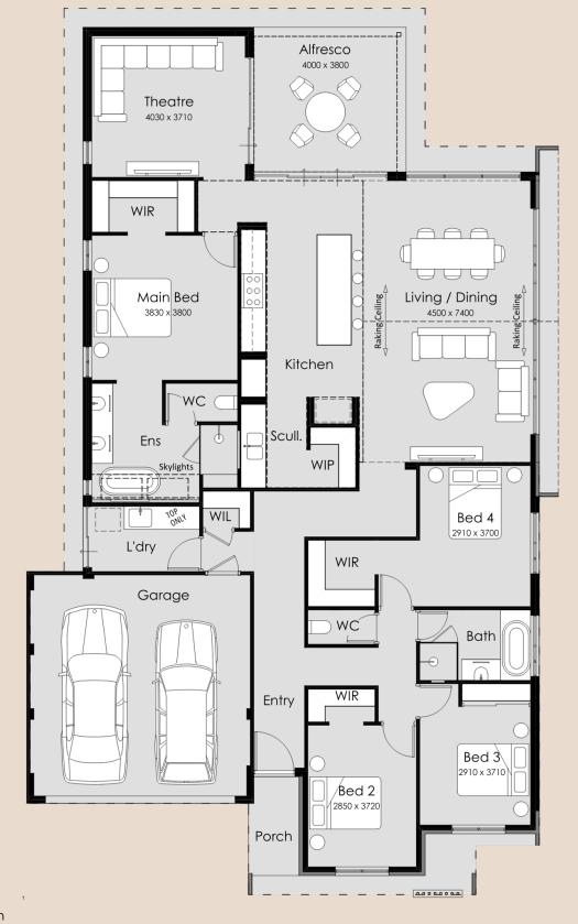
Overall Width – 13.97m Overall Length – 22.79m Min Block Width – 15.00m Min Block Length – 27.00m
