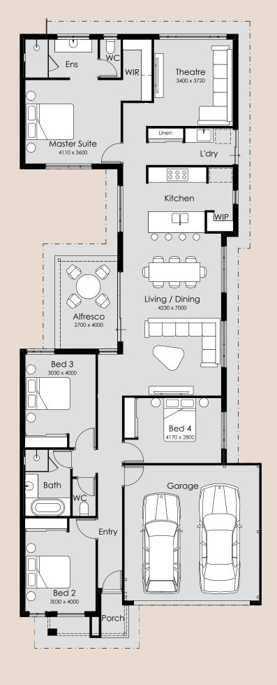
Overall Width – 10.39m Overall Length – 25.89m Min Block Width – 10.50m Min Block Length – 30m Total Area – 213.47m<sup>2</sup>
