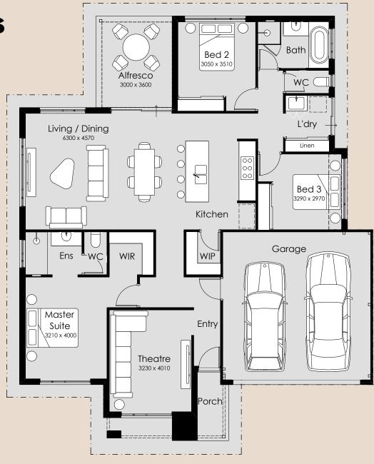
Overall Width – 13.89m Overall Length – 23.69m Min Block Width – 15m Min Block Length – 30m Total Area – 263.82m<sup>2</sup>
