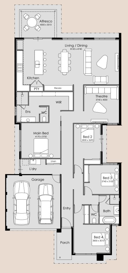
Overall Width - 12.39m Overall Length – 26.70m Min Block Width - 12.5m Min Block Length - 30m Total Area - 256m<sup>2</sup>
